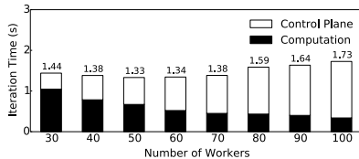
Logistic regression in Spark 2.0 MLlib: Increasingly parallelizing reduces computation time (black bars) but control overhead outstrip these gains, increasing completion time.
